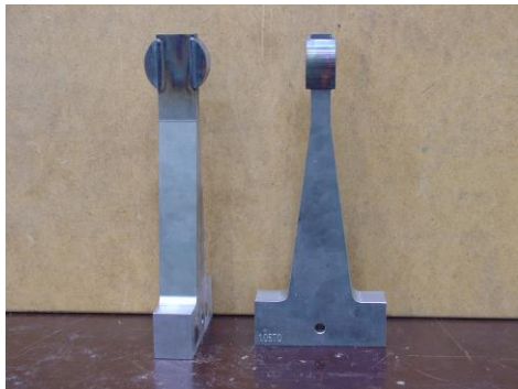
b) TRSH test specimen
