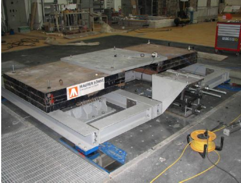
Fig. 11.20: Test mock-up for shake table tests
