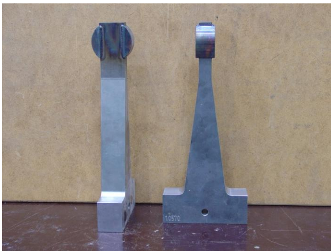
Fig. 11.1: TRSH element with a half-moon head [1]
