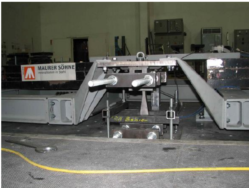
Fig. 11.21: Detail of the steel frame with the TRSH element and its anchoring system
