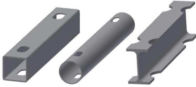
Figure 3.4: Different section types for FUSEIS beam links with reduced beam sections (RBS): RHS or SHS, CHS and IPE- or HEA-section
