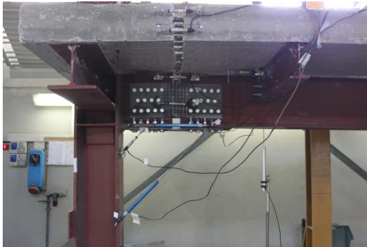
Fig. 5.2: Fuse in a moment resisting frame
