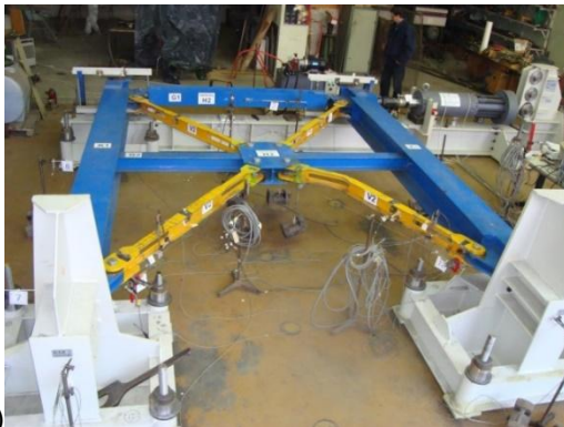
Fig. 9.11: Splitting beam influence, a) unfavourable plastic mechanism; b) bending of splitting beam
