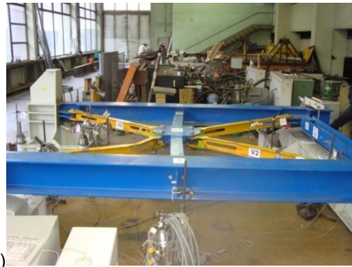
Fig. 9.11: Splitting beam influence, a) unfavourable plastic mechanism; b) bending of splitting beam
