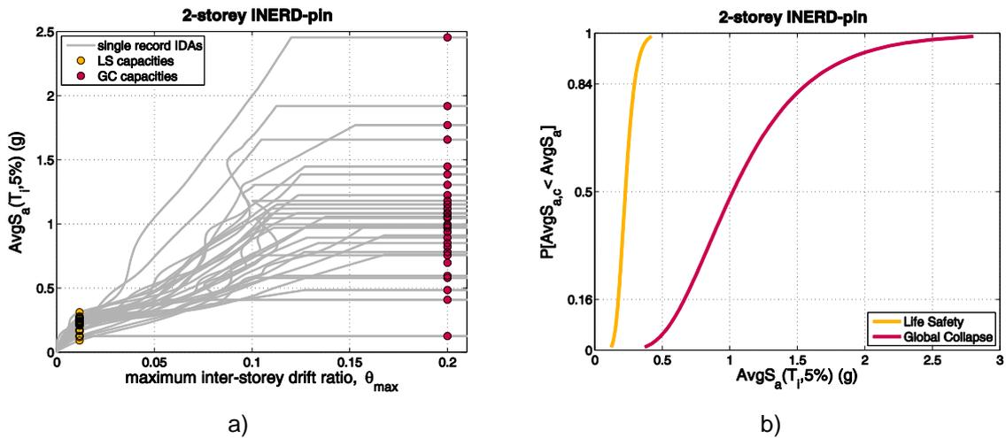
Fig. 2.4: 2-story structure: a) IDA and b) fragility curves
