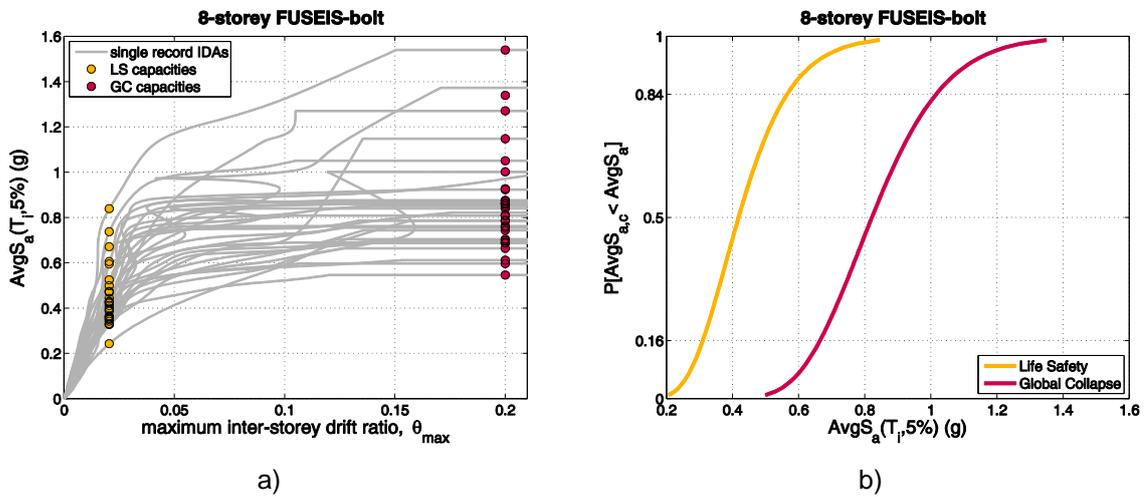
Fig. 6.9: 8-story structure: a) IDA and b) fragility curves
