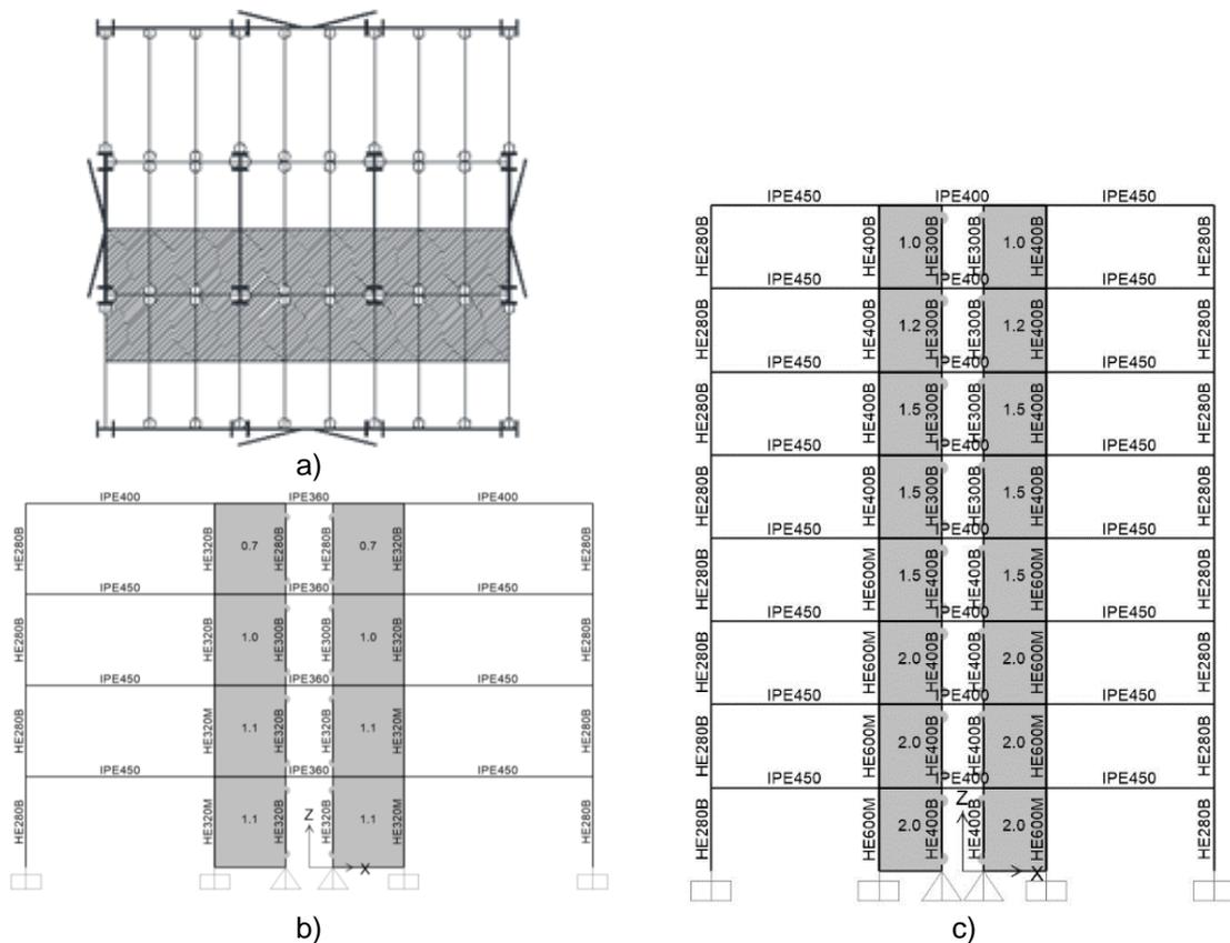
Fig. 9.1: Case-study building frames: a) Plan view, b) 4-story and c) 8-story
