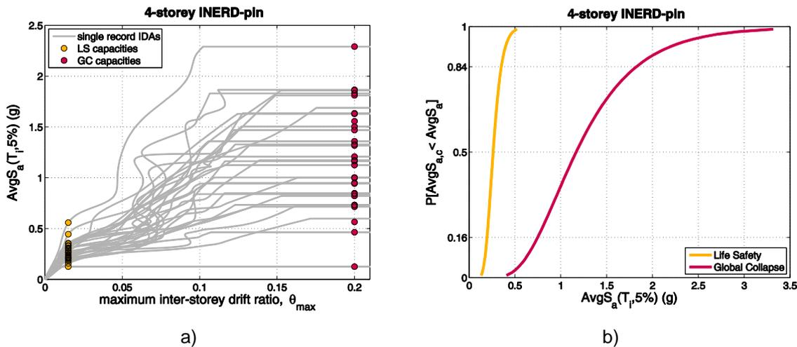
Fig. 2.5: 4-story structure: a) IDA and b) fragility curves
