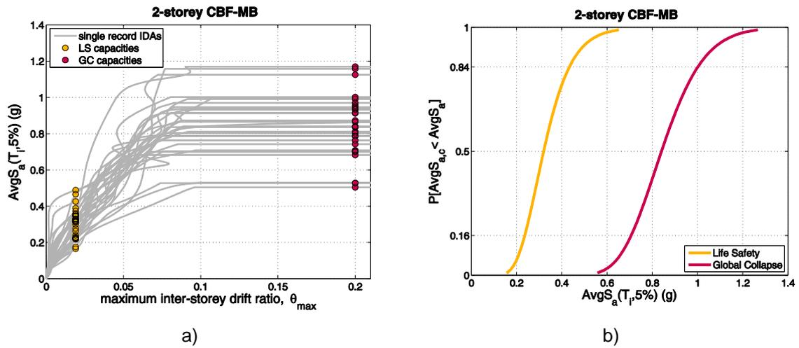
Fig. 10.4: 2-story structure: a) IDA and b) fragility curves
