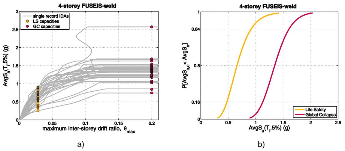
Fig. 7.9: 4-story structure: a) IDA and b) fragility curves
