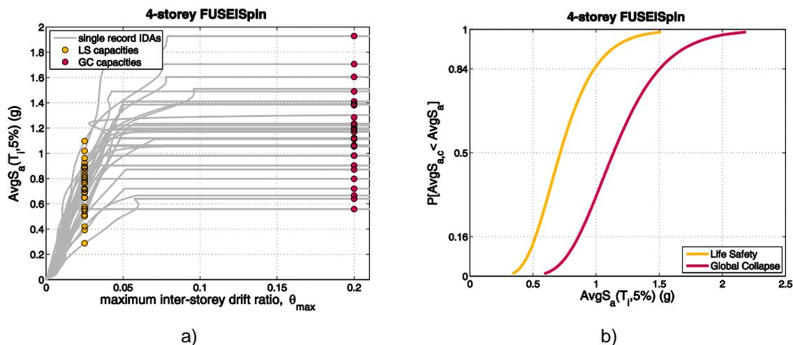
Fig. 5.7: 4-story structure: a) IDA and b) fragility curves
