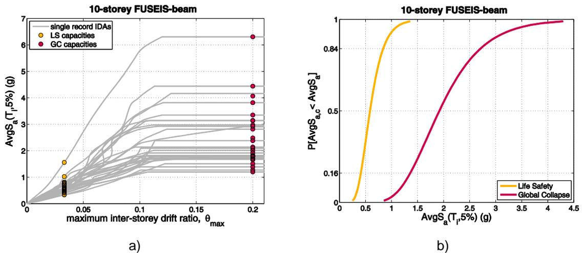
Fig. 4.5: 10-story structure: a) IDA and b) fragility curves
