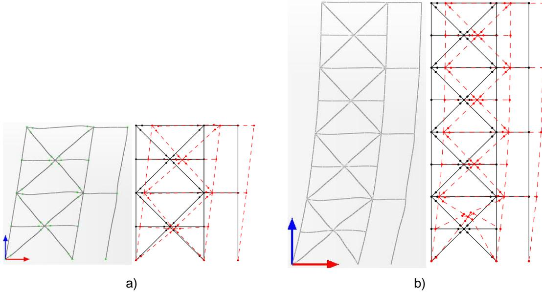
Fig. 10.2: Deflected shapes from SAP2000 and OpenSees: a) 2-storey and b) 4-storey
