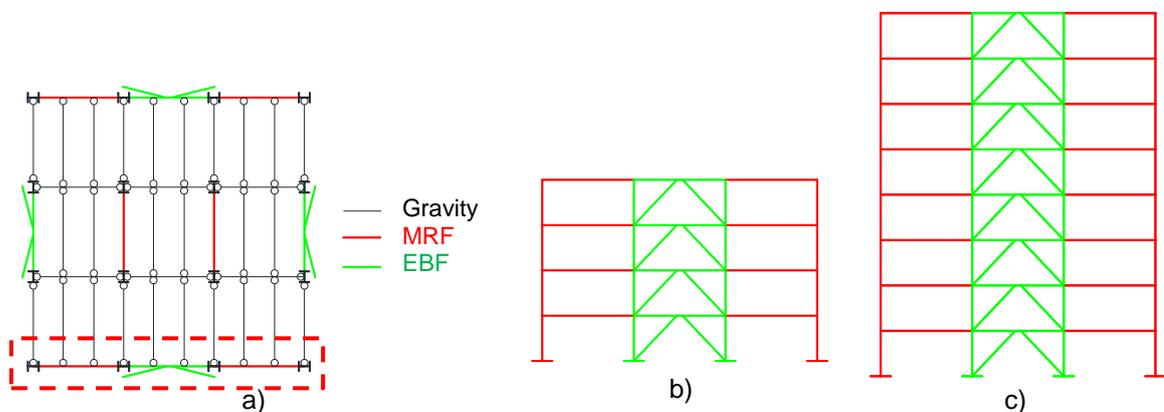
Fig. 8.2: Case-study building frames: a) Plan view, b) 4-story and c) 8-story
