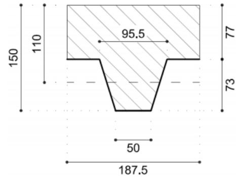
Fig. 7.4: Schematic representation of the composite slab
