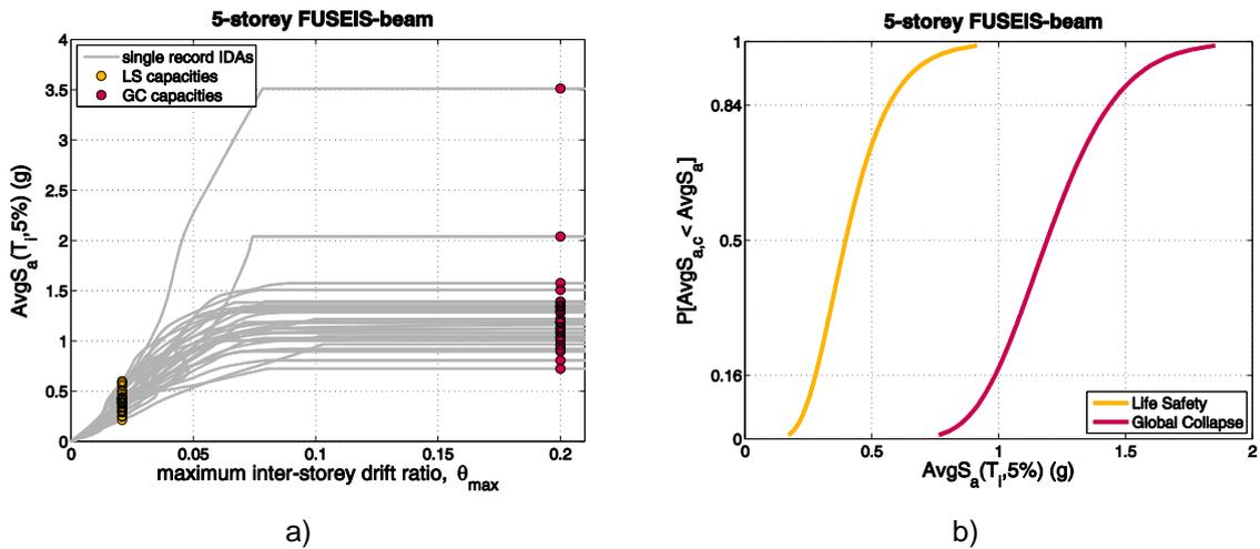
Fig. 4.4: 5-story structure: a) IDA and b) fragility curves
