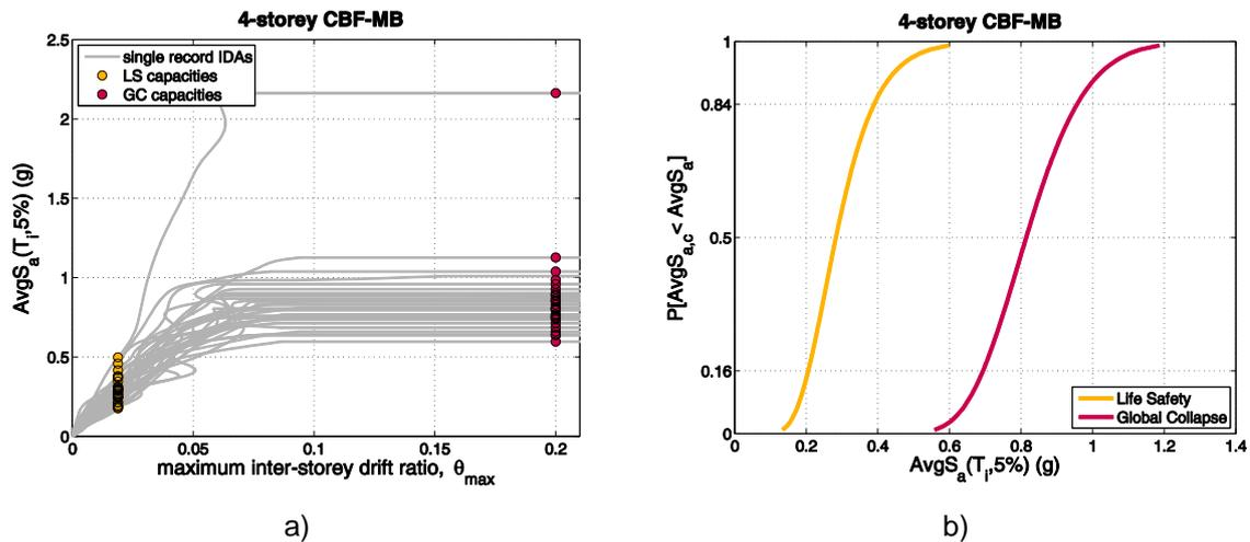
Fig. 10.5: 4-story structure: a) IDA and b) fragility curves
