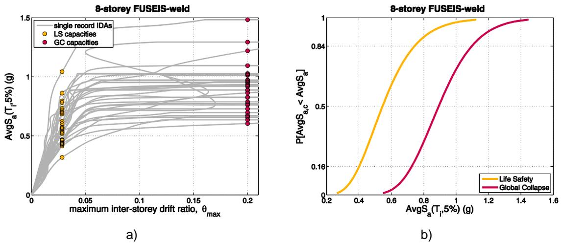
Fig. 7.10: 8-story structure: a) IDA and b) fragility curves
