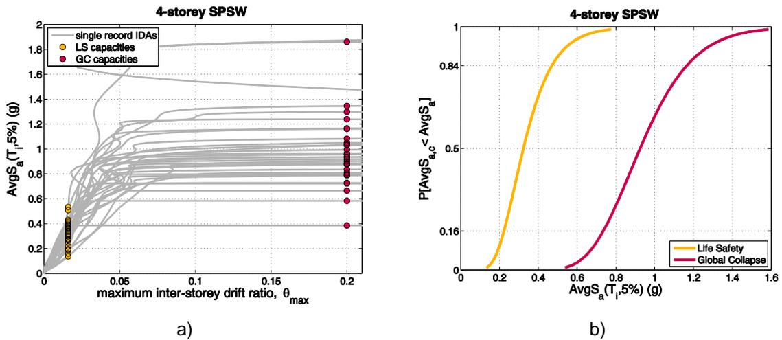
Fig. 9.6: 4-story structure: a) IDA and b) fragility curves
