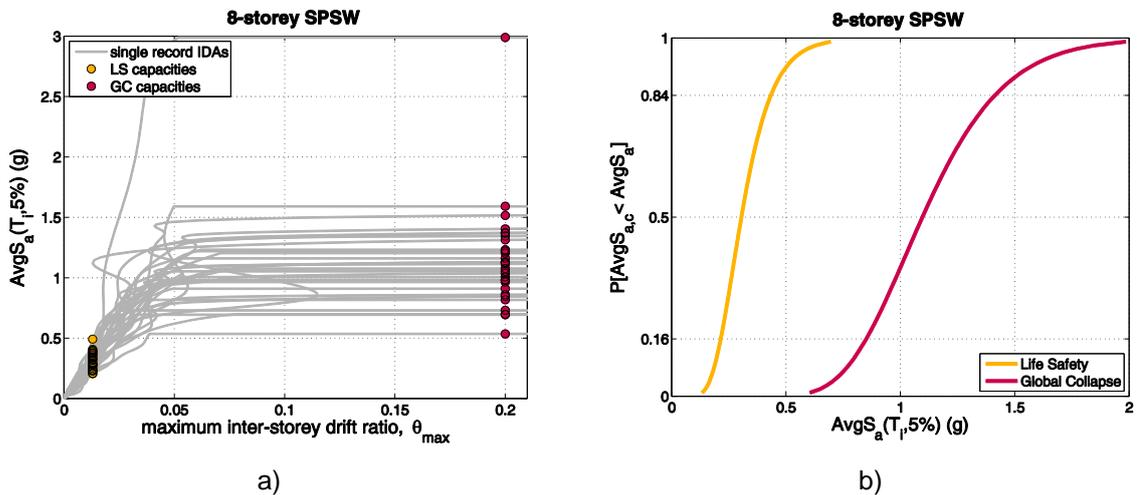
Fig. 9.7: 8-story structure: a) IDA and b) fragility curves
