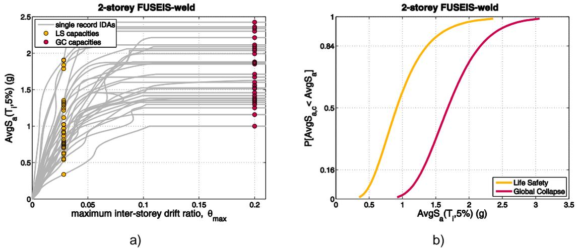
Fig. 7.8: 2-story structure: a) IDA and b) fragility curves
