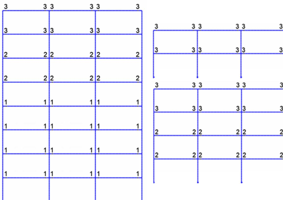
Fig. 6.1: Distribution of assigned bolted beam splices
