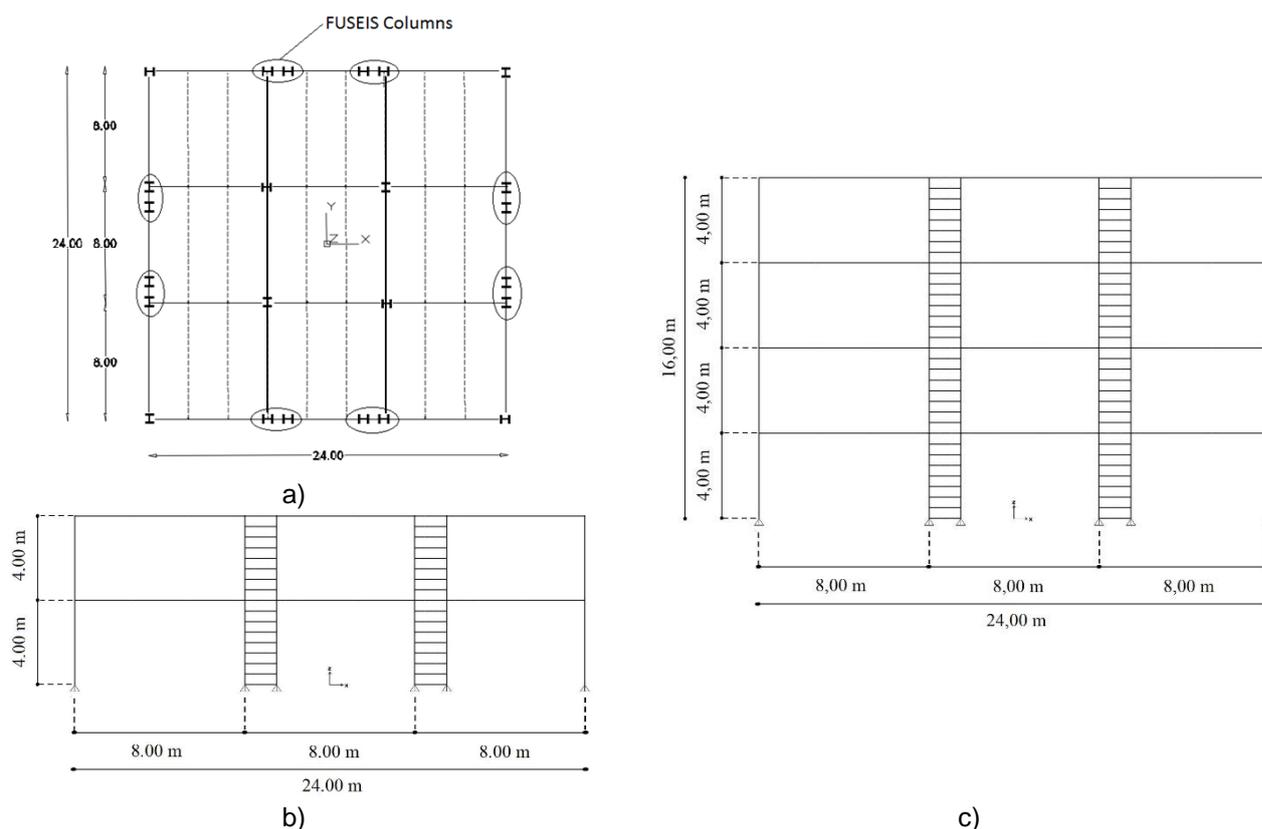
Fig. 5.1: Case-study building frames: a) Plan view, b) 2-story and c) 4-story
