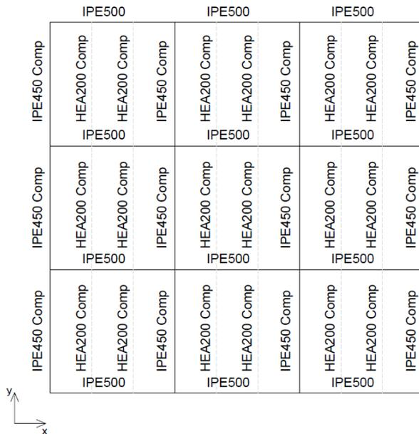
Fig. 7.3: Plan view of the modelled building (the reinforced beam zones and the welded FUSEIS are not represented)
