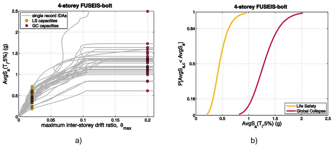
Fig. 6.8: 4-story structure: a) IDA and b) fragility curves
