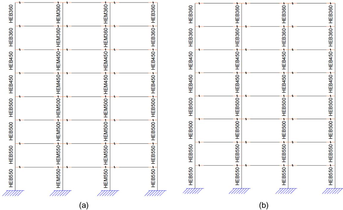
Fig. 7.2: Side view of the modelled building: (a) internal frames and (b) external frames. The reinforced beam zones are highlighted in orange in which the marks that represent the welded FUSEIS can be observed.
