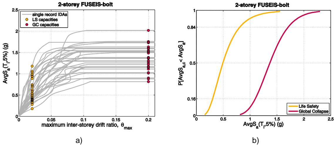
Fig. 6.7: 2-story structure: a) IDA and b) fragility curves
