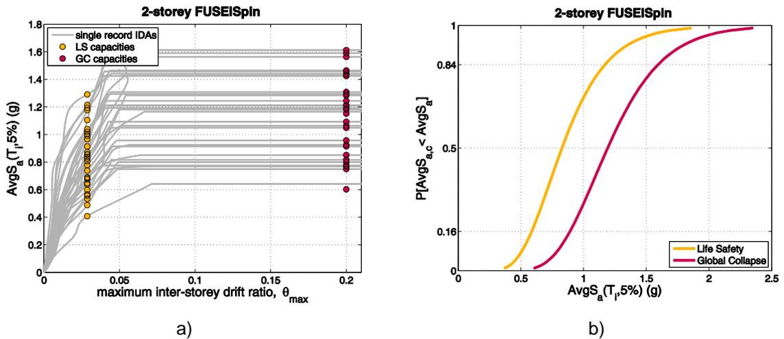
Fig. 5.6: 2-story structure: a) IDA and b) fragility curves
