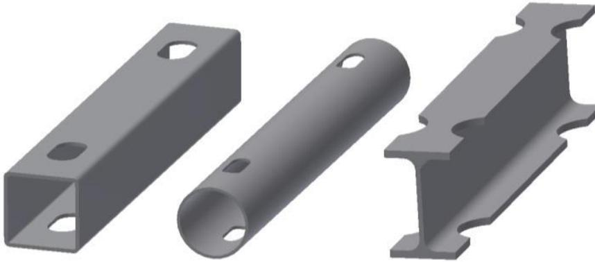
Fig. 4.2: Dissipative zones in FUSEIS beam links by using reduced beam sections (RBS)
