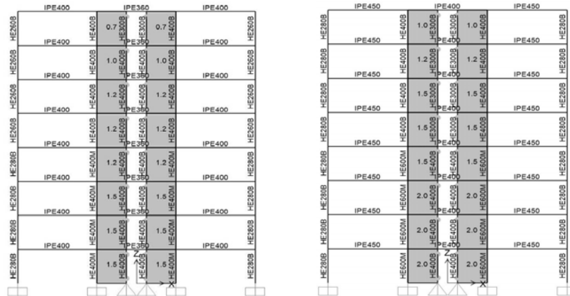
Fig. 11 - 8 story building frames for moderate seismicity case (left) and high seismicity case (right).
