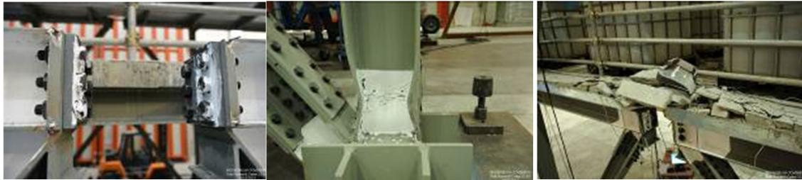
Figure 6. State of the specimen after the last test [3]
