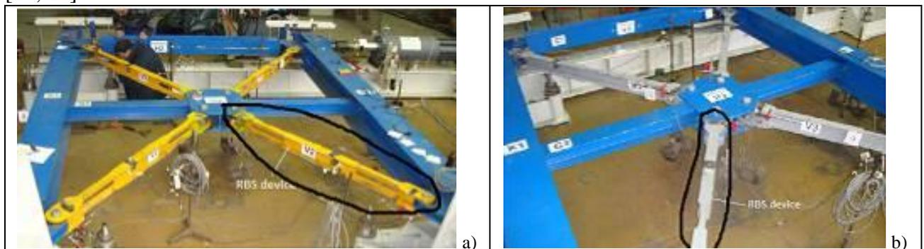
Fig. 6. Modified braces with section reductions at (a) brace ends or (b) the middle of braces
