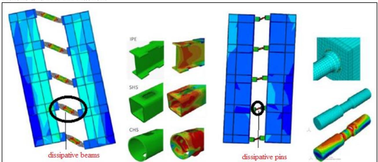
Fig. 2. FUSEIS beam and pin links
