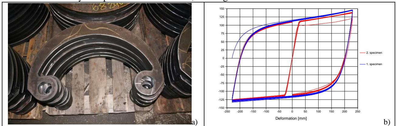
Fig. 9. MSSH: (a) devices; (b) experimental hysteretic curve
