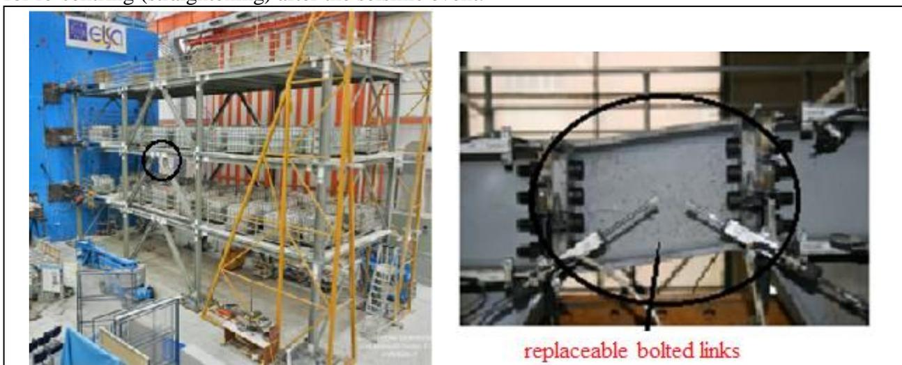
Fig. 4. Large-scale testing of the DUAREM system at JRC Ispra
