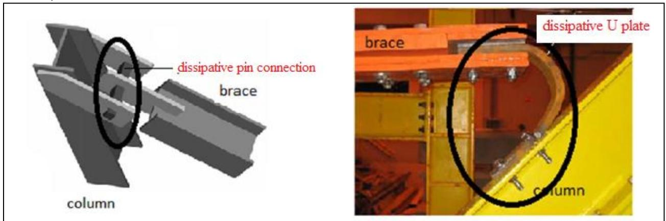
Fig. 1. INERD pin and U connections in concentric braced frames
