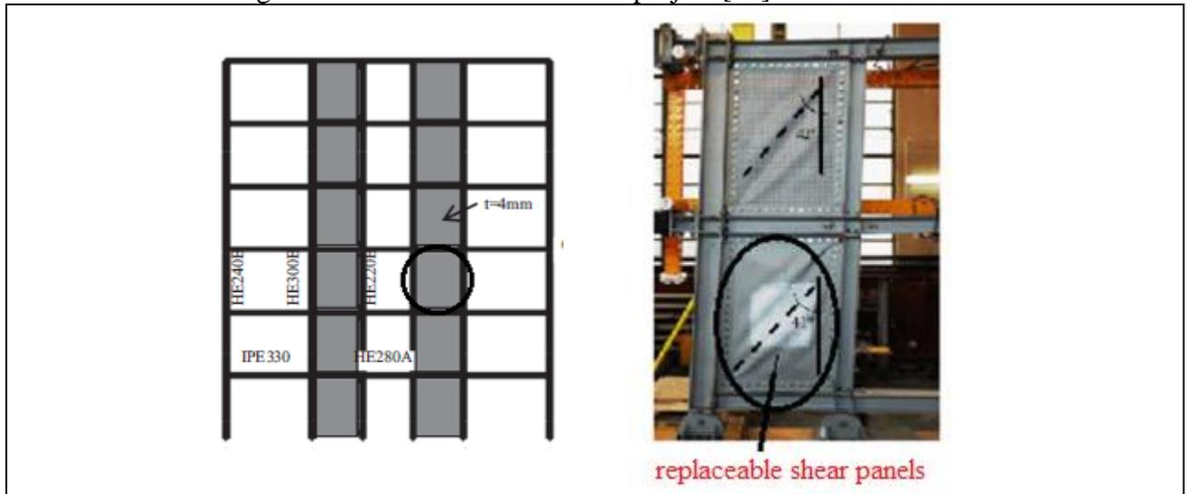
Fig. 5. SPSW replaceable thin-walled shear panel
