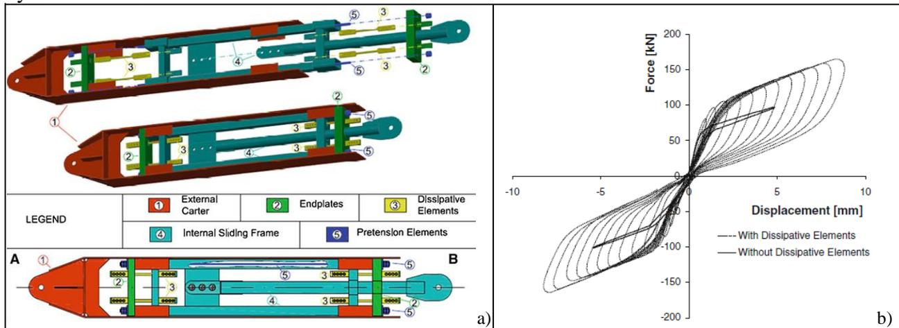
Fig. 7. SSCD: (a) assembling scheme; (b) experimental hysteretic curve
