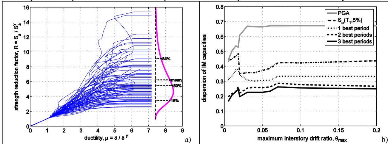
Fig. 10. a) Incremental Dynamic Analysis curves showing global collapse by flattening, together with the distribution of the achieved q-factor, in terms of the collapse fragility (purple line); b) An efficient IM can significantly reduce the dispersion of the fragility function
