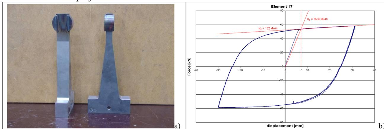
Fig. 8. TRSH: (a) devices; (b) experimental hysteretic curve
